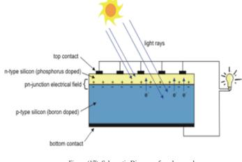
Figure (17): Schematic Diagram of a solar panel.
