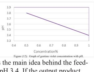
back mechanism. The ideal gentian violet product is of concentration 1% and pH 3.4. If the output product value is larger, the feedback decreases the pH by adding gentian violet, and if the output y = -0.8 x + 4.2value is smaller the feedback increases the pH by adding distilled water to decrease the gentian concentration. Figure (13): Equation of relation between pH and concentration
